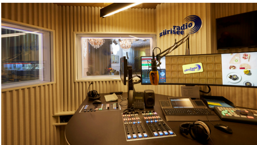
Radio studio workplace with smartTOUCH keyboard, smartVISUAL personal videowall and an integrated mixing console
