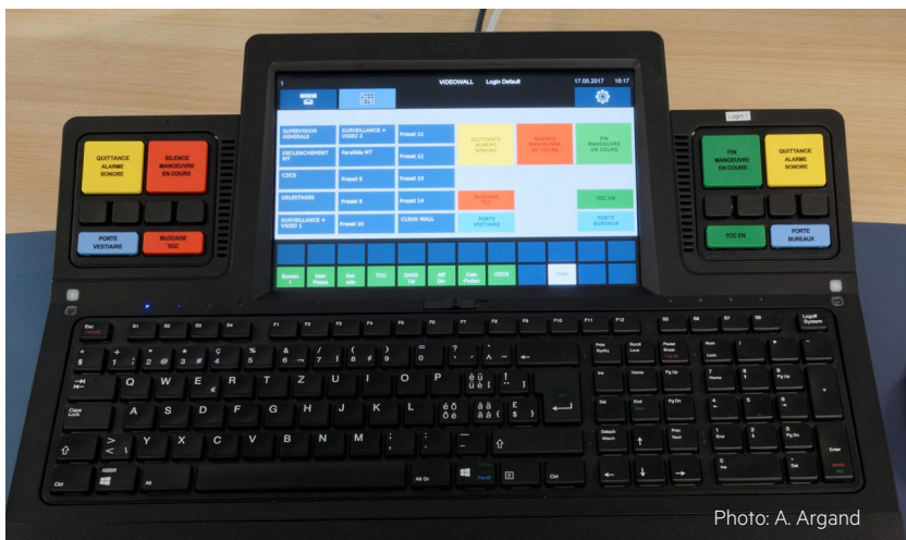
WEYTEC smartTOUCH: The multifunctional keyboard with customized key pads to the right and left of the keyboard screen.
