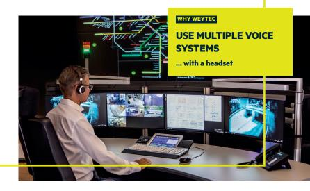
LAPS (Local Audio Processing and Switching) consists of an audio DSP, a voice switching controller and operating software. It switches, mixes and outputs a variety of analog and digital audio signals from telephones, Polycom, analog radio and PC sources. The system is operated directly at the workplace via the WEYTEC smartTOUCH keyboard touch screen.
