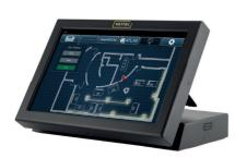
The touchscreen provides a user-friendly interface to work with diverse systems. It displays all sources and monitors. Available sources are indicated in green, occupied sources in red and «view only» sources in white. Sources are easily selected and assigned to monitors and video walls. Switching between individual sources is simple using tabs.
