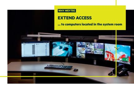
The WEYTEC point2POINT solution deploys IP-based KVM extenders to transmit keyboard, video, mouse and audio signals on a point-to-point basis. PCs and other information sources are removed from the desk and housed in centralized system rooms where they are secured, maintained with simple and efficient workflows and cooled cost-effectively. In addition, up to 16 PCs can be controlled with a single standard keyboard and mouse using additional USB deskswitches.
