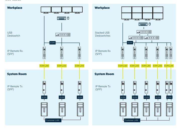
IP Remote components can be used in a point-to-point environment to extend keyboard, mouse, video and audio signals.
